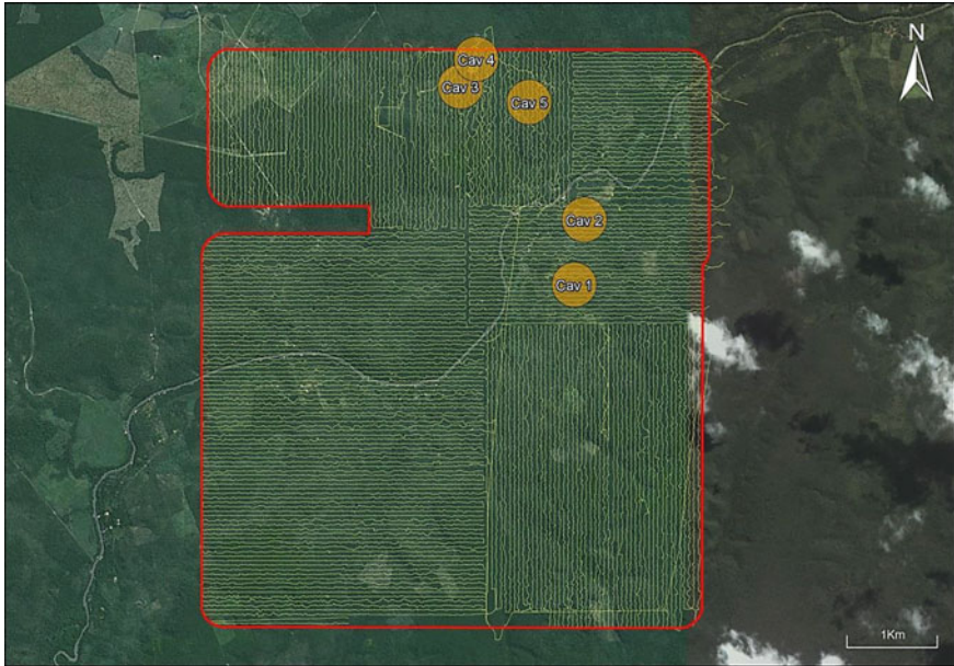
Fig. 2 GPS-equipped cave-prospecting teams of 2–3 members walk alongside one another, creating 50 m-wide parallel lines that represent the walking route. Line spacing depends on cave potential and visibility (which varies with rock type, vegetation and relief). Ideally, spacing equals the distance of visibility/2. Areas between lines may be checked if necessary. Areas containing high-potential features such as dolines and rock outcrops must be inspected in more detail. Orange circles denote a 250 m buffer zone of identified caves
